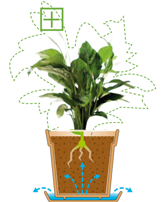
water reservoir and wateroverflow helps the plant grow
